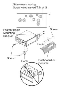
To fasten the unit to the factory radio mounting brackets.
